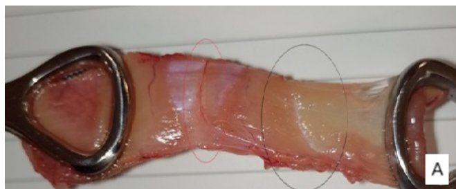
Figure 3. Specimen detail after rupture. A: Detail of the specimen after rupture at the semilunar line. The red circle marks the midline (no rupture), while the black circle marks the semilunar line (ruptured). B: Detail of the specimen after rupture at the midline.
