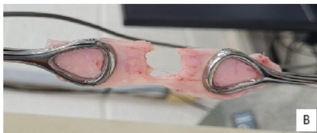
Figure 3. Specimen detail after rupture. A: Detail of the specimen after rupture at the semilunar line. The red circle marks the midline (no rupture), while the black circle marks the semilunar line (ruptured). B: Detail of the specimen after rupture at the midline.
